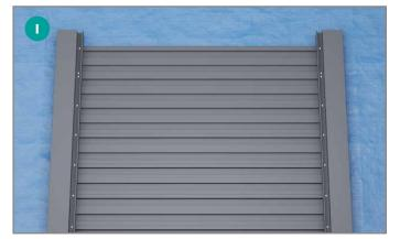
Repeat installation of the remaining Slats securing with a self-drilling screw 12mm from the top edge of the profile on either side, ensuring that the assembly is on a protected level surface whilst doing so.
