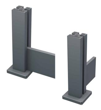
Then using a 4mm drill bit and a cordless drill, drill a pilot hole through the drill line in the front centre of the post for the self-drilling screws 50mm above the base plate and then at 100mm centres going up the post. Ensure you have a minimum of 4 fixings per post and the screws are in the centre of the channel.
