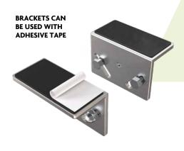
Designed to provide an economical but versatile pedestal option, our 6mm thick Jumbo Adjustable Pedestal Brackets are A1-rated and noncombustible as they are manufactured and supplied in mill-finish. Simple but highly effective allowing users to create an even greater build up height. Installation and levelling can be accomplished quickly and easily with the L-shaped aluminium brackets with sloping bolt channels.
