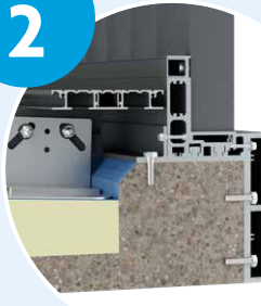
Vertical Infill Balustrade: Concrete Fix 0.74kN Option
