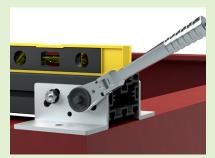
STEP 8: Check the level again and fix to your sub-structure through the base of the Adjustable Pedestal Brackets
