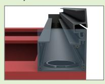
Lay the first decking board, overlapping the Gutters but allowing 1-2mm clearance to the Access Lid
