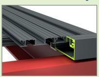
STEP 10: Run a bead of Sikaflex sealant along the exposed side of the Drainage Channel
