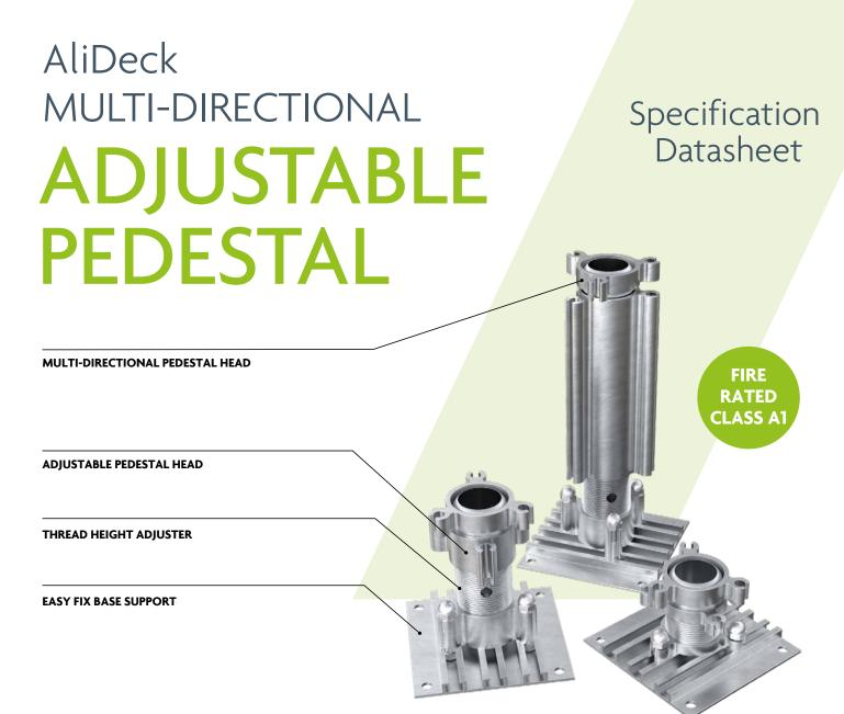
The AliDeck Multi-Directional adjustable pedestal is a solution driven product, specifically designed for installations where you need a multi-directional foot position due to a fall 2 or more ways in the floor. This solution is perfect for insulated roofs (with or without membranes) which are laid to fall, they can bolted or bonded using our fire retardant double sided tape.
