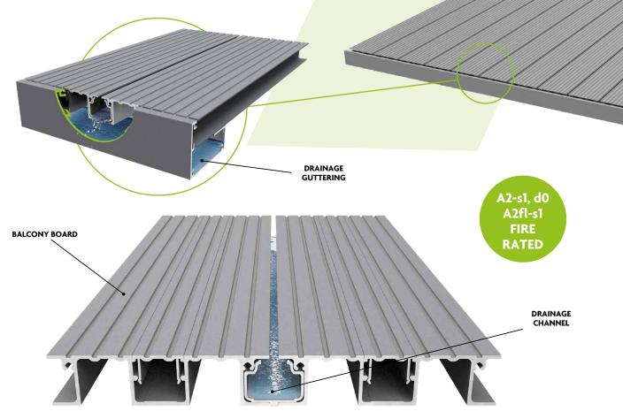
This discrete extrusion is installed between the balcony boards to aid with drainage and reduce the flow of water between the boards, available for the 20mm & 30mm balcony boards, it may reduce the need for expensive soffit claddings on balconies.
