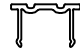
Senior Balcony Flat Board Clip Maximum length 6000mm Can be joined SCALE 1:1
