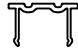
Junior Balcony Flat Board Clip Maximum length: 6000mm Can be joined SCALE 1:1
