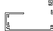
Junior Balcony Board Gutter Channel Maximum length: 6000mm Can be joined SCALE 1:1
