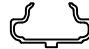
Junior Balcony Board Drainage Channel Maximum length: 6000mm Can not be joined SCALE 1:1
